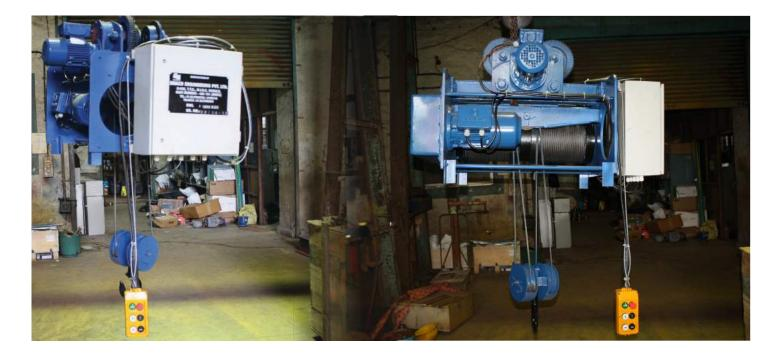
Flameproof Wire Rope Electric Hoists are generally used in oil & gas industries, chemical industries or in hazardous areas where explosion is possible due to mechanical/electrical sparking; for gas groups IIA/IIB & IIC.
