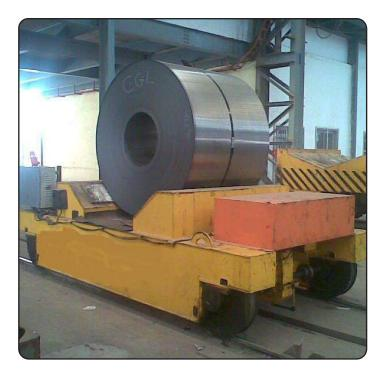
We are a well established manufacturer and exporter of Transfer Trolley. Our products are manufactured using standard quality materials and advance techniques. The offered range of Material Transfer Trolley are available in varied sizes to cater to the diverse requirements of our esteemed clients. Apart from lifting transformer, it can move transformers from one place to another. This model does not incorporate any pallet.
