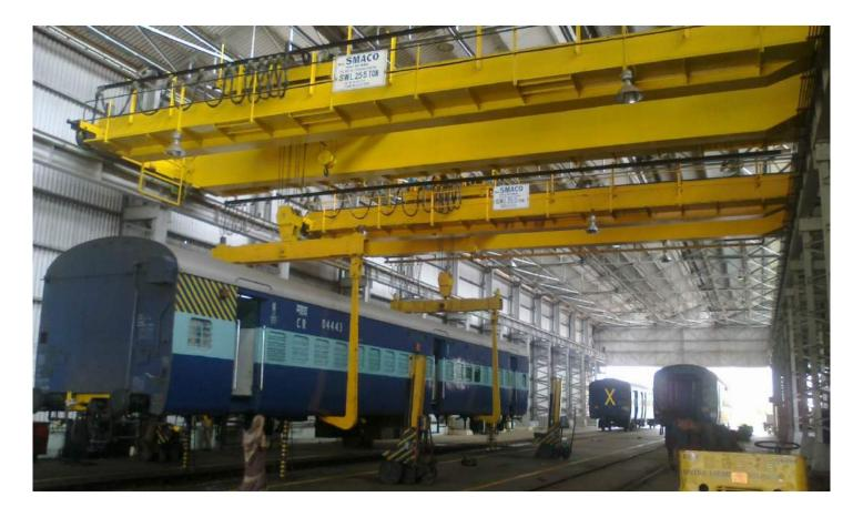
We are among the prominent organizations engaged in manufacturing and supplying superior quality Double Girder EOT Crane. These cranes are used for material handling and are best suited for both medium and heavy duty operations. These kind of Cranes are generally used when heavy loads and wide spans are needed. These double girder EOT cranes are widely used in all types of industries.
